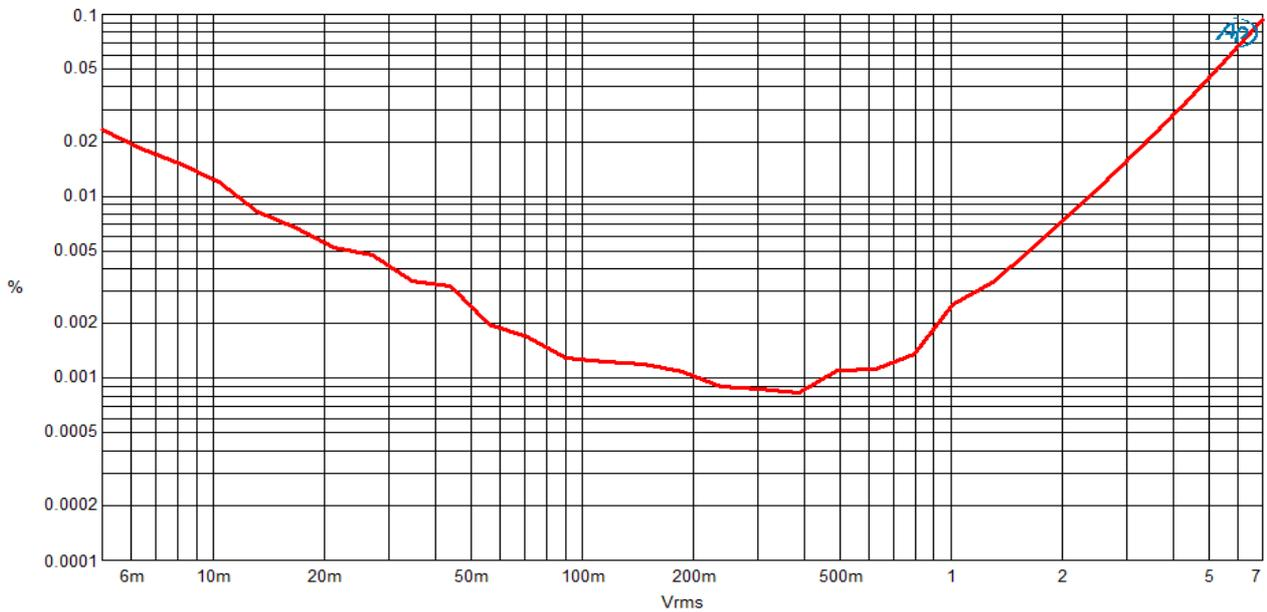
Fig.4 THD vs. level at 1kHz and 10k load
