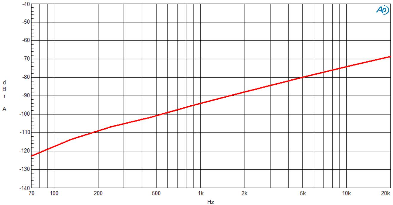
*Fig.10 Cross-talk into adjacent channel at 8V into driven channel. 10 k load.*
