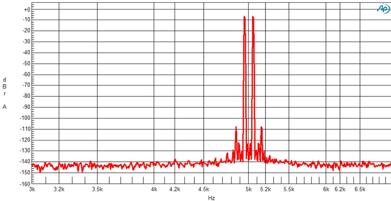
*Fig.8 CCIF IMD test, 19+20kHz, -6dBV, 10k load*
