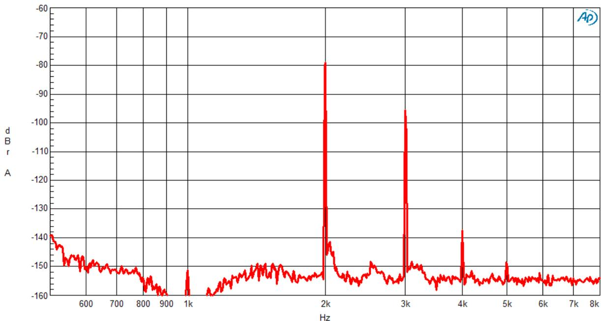
*Fig.1 THD at 1kHz, 1V, balanced, 10k load*
