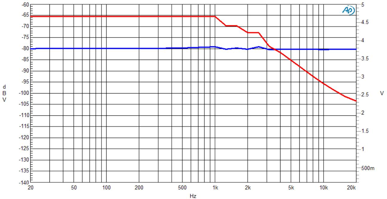
Fig.9 Max. input level vs frequency for 0.01% THD+N
