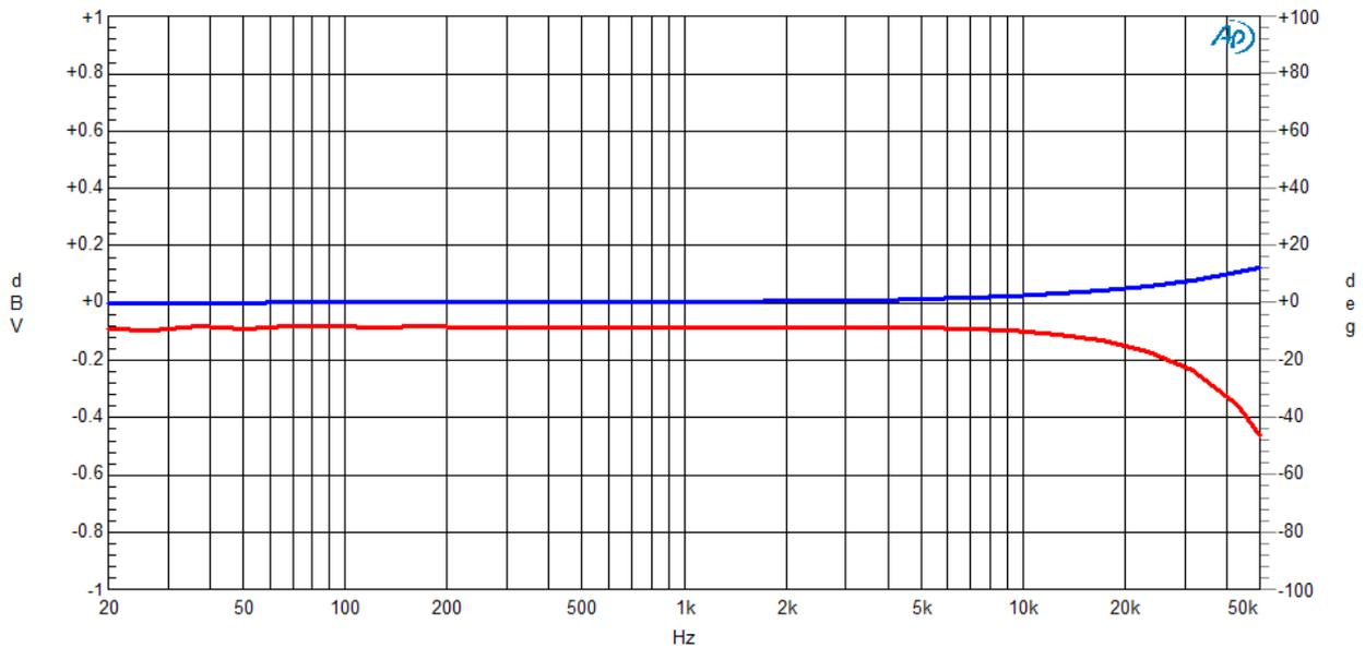
Fig.6 Frequency (red) and phase (blue) response at 1V and 10k load
